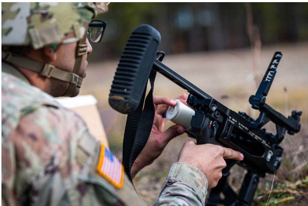
Above: An instructor with the 1-114th's Charlie Company instructs a Soldier during M320 grenade launcher training. The M320 replaced the M203, which first saw service in 1969. The M320 is designed to operate both as a stand-alone weapon, in addition to being mounted to the M16 rifle
